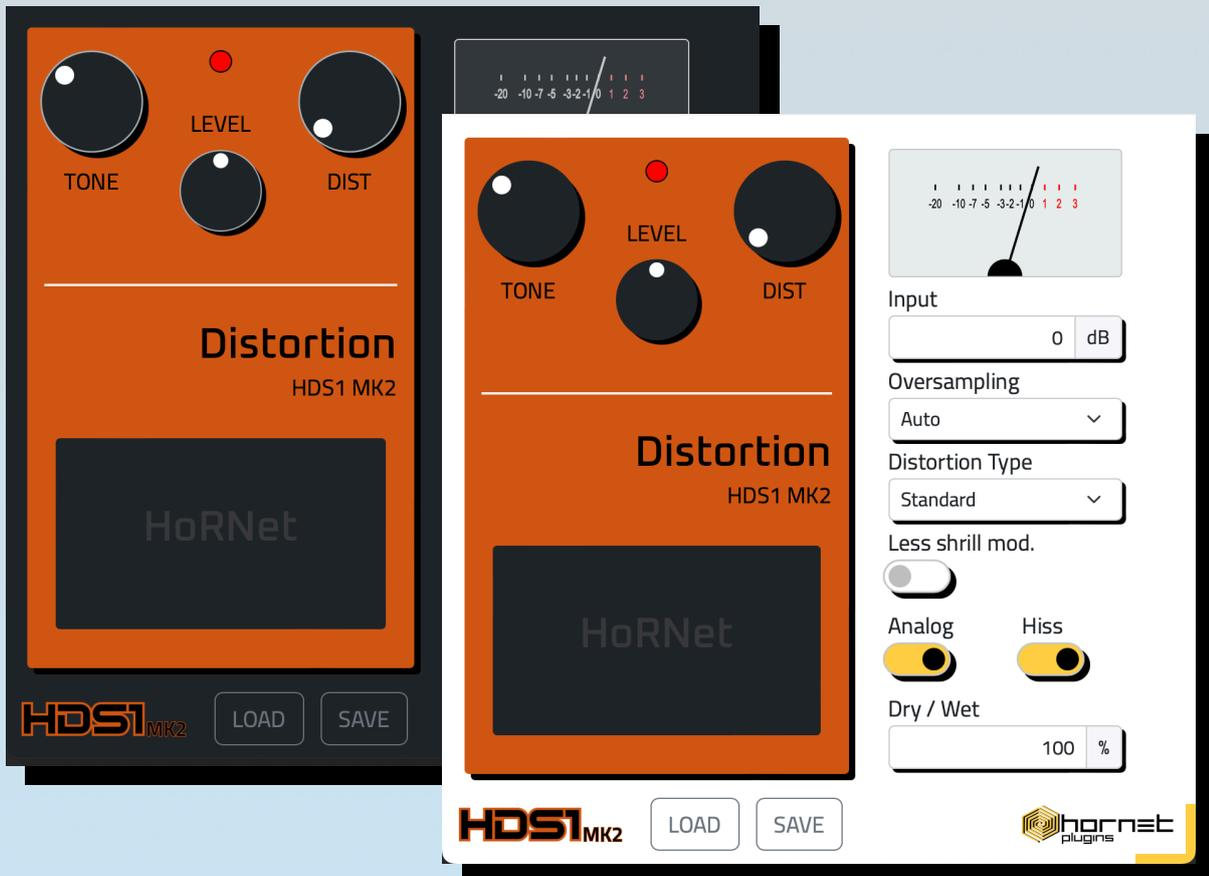
The **HDS1 MK2** core is made by three different stages: a simple **transistor boost**, a **dual op-amp amplifier** and a **diode clipper**. The first stage shapes the frequency response by boosting the higher frequencies; the second stage enhances the gain for the clipping stage and provides a variable lowpass filter modulated by the gain amount (increasing the gain lower the cutoff point). Finally the diode clipper brutally limits the signal and adds the hard distortion.
